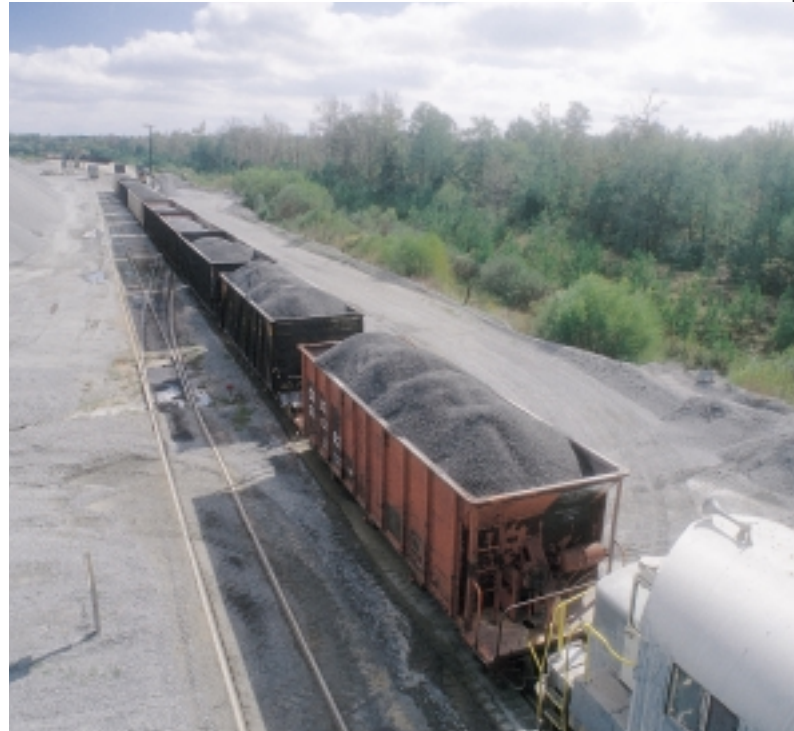
Junction City quarry ships the majority of its 2 million-ton annual production via railroad to customers as far away as 250 miles. A significant amount of product from this location is used by the railroad for ballast.
